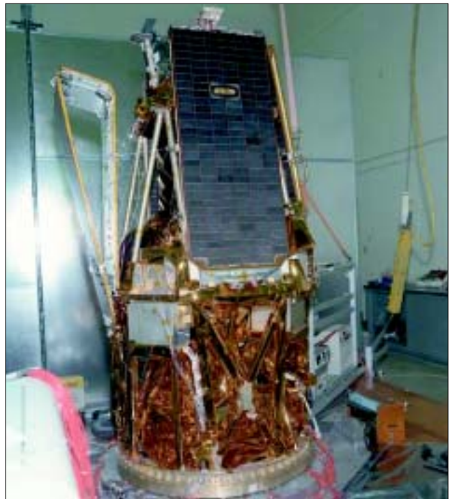
Figure 15. HESSI solar array damage.
