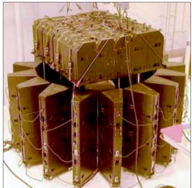
Figure 11. COTE direct acoustic test.
